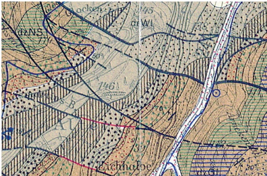
Figure 5: Geological map from 1957, area between Hahnenklee and Goslar with the highway B241,  $51^{\circ}52'16.46''N$   $10^{\circ}23'10.33''E$ . The main lines of the projection pattern (black) extend approximately from east to west. Pay zones are indicated in red.
