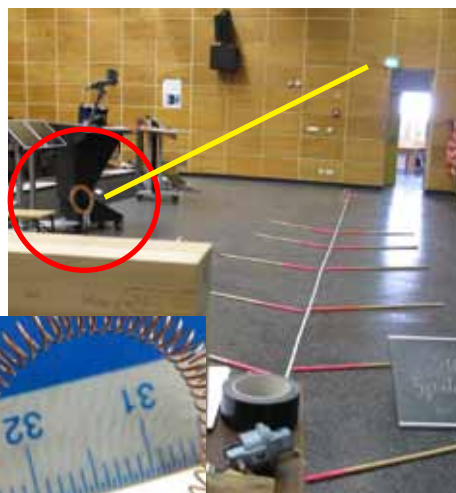
Fig. 16: The beam of a HeNe laser lights on the wall in the background. Along the beam are periodic structures to be detected.
