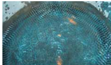
Fig. 10: Standing waves in a singing bowl by periodic motion of the vessel walls.
