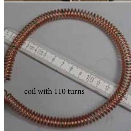
Fig 20a. 20b; 20c: the three coils with 28; 60 and 110 turns
