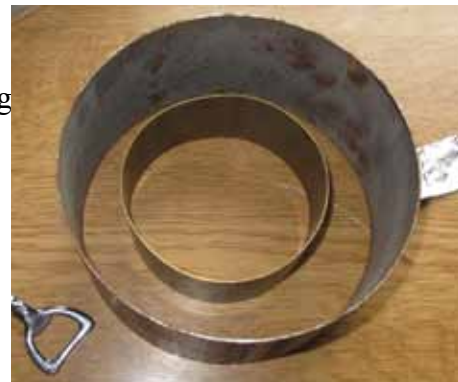
Fig. 07: Two hollow bodies made of different materials: brass and iron. Right a small wire connects the two bodies together electrically.
