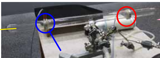
Fig. 14: Gas discharge tube. On the right side (cathode) something can be perceived with the palm outside the Duran glass tube slightly to about 1.5 meters.
