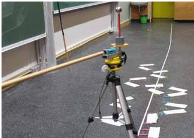
Figure 32a. 32b: At the stage of the lecture hall, the turntable is rotating with the hollow sphere. Right: metal ball in front of the electrodes of the "Feldmuehle" (E-field meter). Paper and colored chalks on the ground mark the positions of significant structures. There are four marks per charge voltage. ( / \ / \ )
