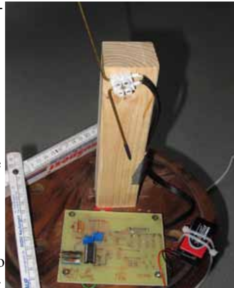
Fig. 38: turntable with small dipole. The dipole axis is inclined to the rotation axis and stumbles upon rotation of the plate. The small generator is battery powered and rotates on the plate with.
