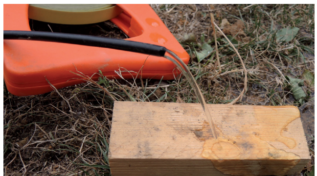
Figure 16: Reproduction of the experiment depicted in figure 1 with a simple construction: Crossing of two hoses at different heights, low flow rate of water; low pressure, 5 mm inside diameter. The perceptible effects due to the influence of electrical devices are similar.
