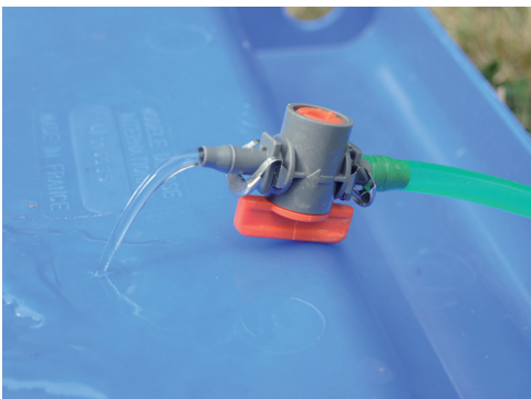
Figure 16: Reproduction of the experiment depicted in figure 1 with a simple construction: Crossing of two hoses at different heights, low flow rate of water; low pressure, 5 mm inside diameter. The perceptible effects due to the influence of electrical devices are similar.
