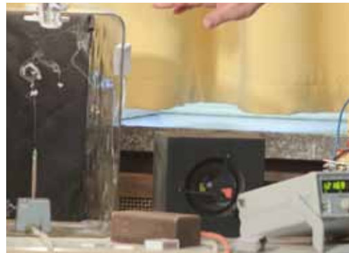
Fig. 29: The smoke tubes (left) were periodically blown through a hose by a swinging speaker cone (center). The frequency was adjustable.
