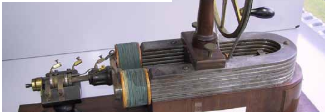
Fig. 08: Induction coil (alternator) from the 19th century, built among others reasons for medical purposes by the Dr. Stöhrer Company in Leipzig. The horseshoe magnet consists of seven layers of forged iron. / Balck 2011 /
