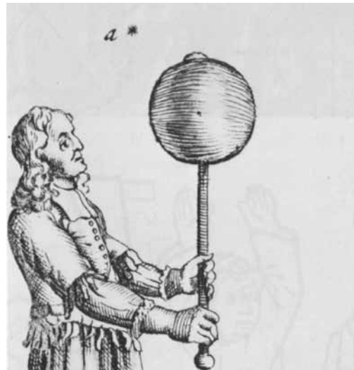
Fig. 01: Charged sulfur ball, Otto v. Guericke, 1672, bird feather (a) is repelled. / Teichmann 1996 /
