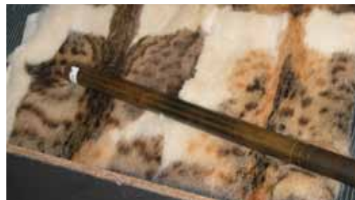
Fig. 02: Static electricity with catskin and plastic rod (resin) Charging negative (resin electricity)
