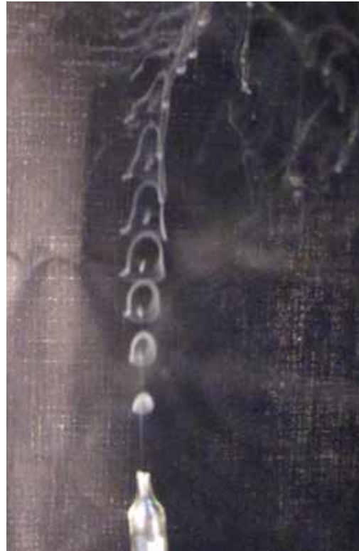
Fig. 28: Similar structures were produced using a periodically-blown smoke tube usually used to detect air flow.
