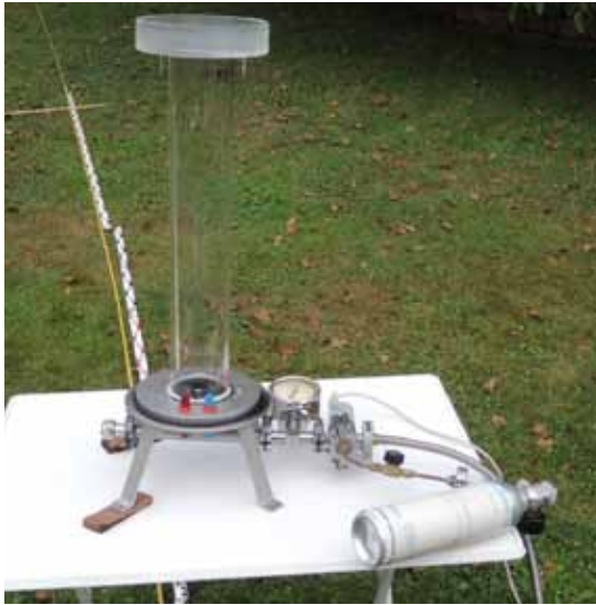
Figure 30: The quartz tube has been sealed air-tight above and below, and can thus be evacuated. By means of an appropriate filling device, the tube can then be refilled with gas. (An aluminum cylinder containing neon is illustrated in the figure.)
