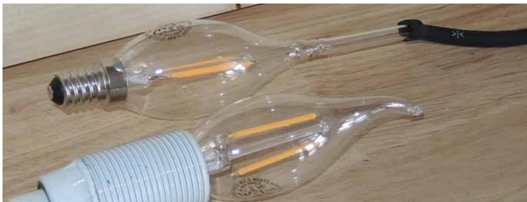
Figure 37: Retrofit LED lamps have a glass envelope which is filled with a special gas for improving the heat dissipation. If this gas is pumped out and replaced by carbon dioxide, the perceptible effect which is observed during the operation of these lamps can be suppressed.
