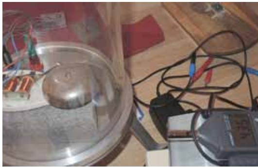
Figure 26: (left) An electromagnetic door-bell is placed in a vacuum chamber. A sound-level meter is located on the right-hand side of the chamber.
