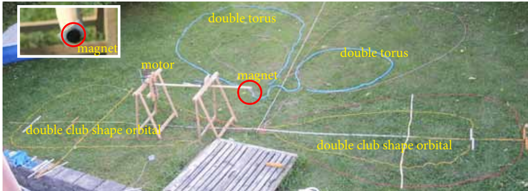
Figure 22a: (left) A flat bar magnet has been cemented to the tip of a wooden pole.
