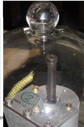
Figure 28: (r.m.): A flat neodymium bar magnet is mounted on the shaft of a motor. Both are located in a vacuum chamber.
