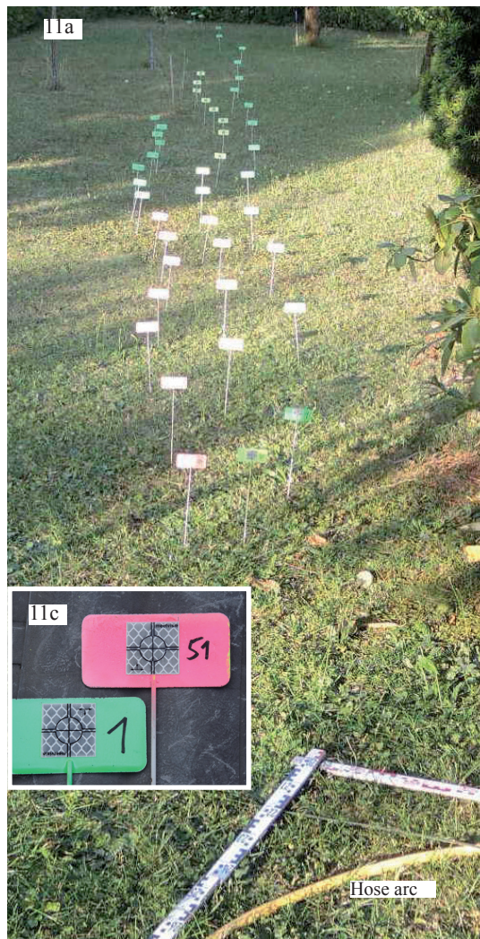
Figure 11a: Bend in a hose with measuring stick: Three rows of reflector marks in the background correspond to three different velocity values. The respective marks identify one point on each ring. The period is shorter for the left-hand row and longer for the right-hand row.
