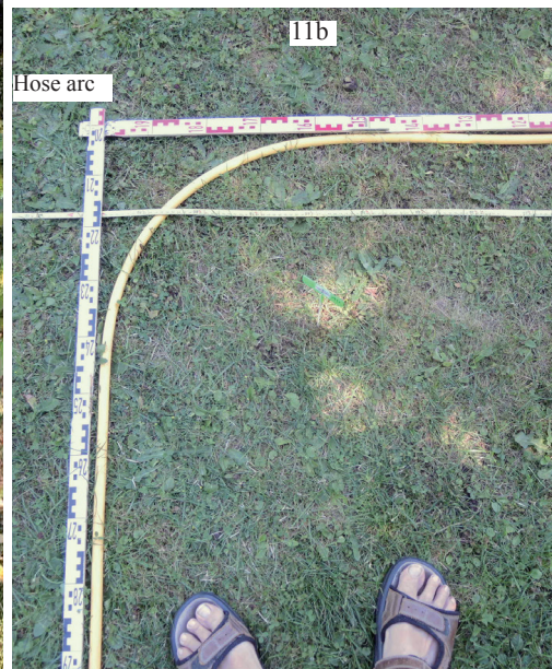
Figure 11a: Bend in a hose with measuring stick: Three rows of reflector marks in the background correspond to three different velocity values. The respective marks identify one point on each ring. The period is shorter for the left-hand row and longer for the right-hand row.
