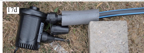
17d: Fan for inflating air mattresses with electronic unit for controlling the rotational speed
