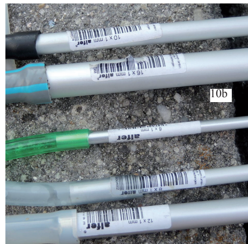
Figure 10: Different diameter and materials 10a: from left: black PE inside diameter 5 mm, plastic pipe for domestic installation, 40 mm, connected with a PVC hose, inside diameter 6 mm; yellow 1/2" hose; right: aluminium pipes with 1 mm wall thickness 10b: Outside diameter: 16, 12, 10, 8, and 6 mm; flow rate for experiment: 0.180 litre/minute
