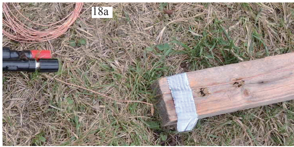
Figure 18: A copper wire with a diameter of 0.6 mm lies on a wooden board in the north-south direction.
