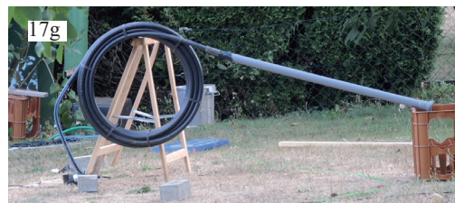
17f and 17g: Coil of 20 mm plastic (HDPE) pipe, left with flowing water, right with flowing air
