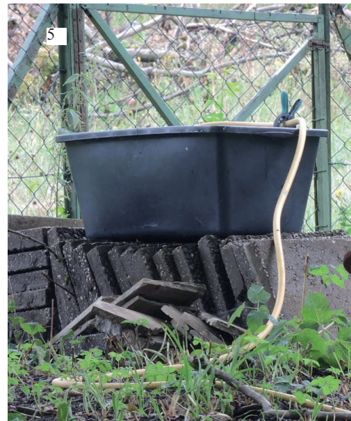
Figure 5: A small elevated storage vessel is sufficient for the experiments. After priming by suction on the hose, the water flows out independently. At the low flow rates in the range of litres per minute, the supply of water is sufficient for experiments of long duration.
