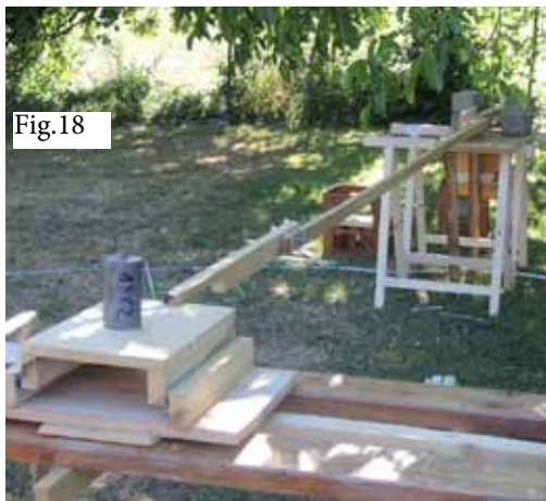
Figure 18: Iron cylinder mounted on a translation stage driven by a crank mechanism by way of a long wooden pole
