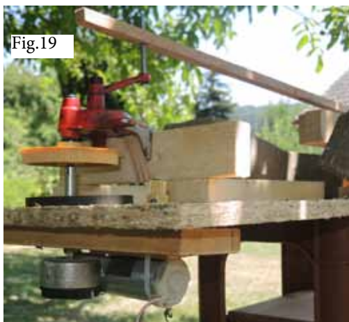
Figure 19: Electric motor with transmission gear, crank mechanism, and wooden pole
