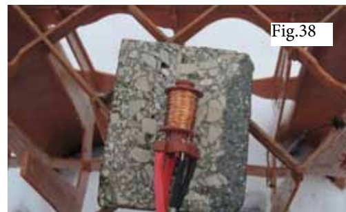
Figure 38: A copper coil with a ferrite core on a concrete block, the end point of a sixpack
