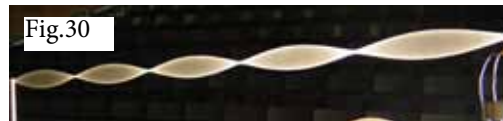
Figure 30: Waveform resulting from an increase in the length of the cable or in the excitation frequency by a factor of 5/2, in comparison with the left-hand figure
