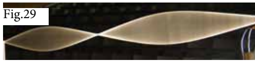
Figure 29: Periodic excitation of an elastic rubber cable at one end by an eccentric motor and generation of standing waves at the corresponding frequencies (appearance of the cable motion as a pale surface as a result of smearing because of the long exposure time)
