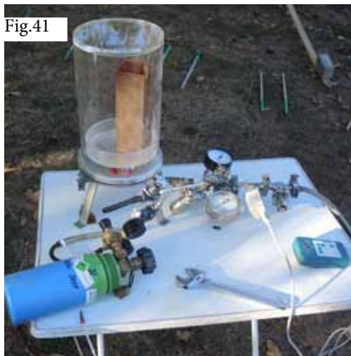
Figure 41: Vacuum chamber with devices for filling with noble gases: helium, neon, argon, krypton, and xenon: The target for a psi track, the copper sheet depicted in figure 14, is in the vacuum chamber.
